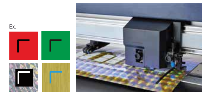
* Sensor may not be able to read certain combinations of specialty media and colored marks.
